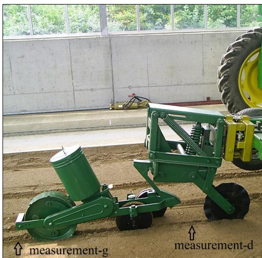
Figure 7. Experimental prototype with rifle disk
