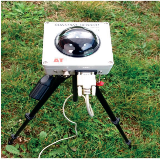
Figure 4. Beam fraction sensor (BF2) used simultaneously with a Quantum Sensor (QS) connected to a DL2e data logger (Delta-T Devices) for PAR multilayer measurements ( \mu\text{mol m}^{-2} \text{s}^{-1} ) in the canopy
