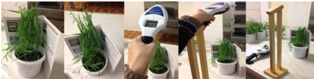
Figure 4. Measurements taken by GreenSeeker Handheld Crop Sensor (Trimble) on wheat seedlings
